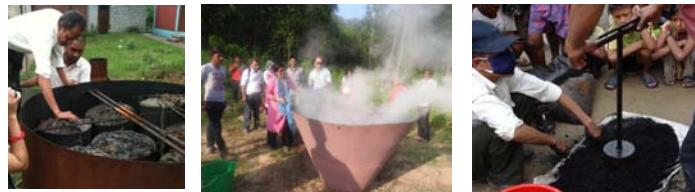
Charring different kinds of Biomasses to convert into biochar and biobriquettes
