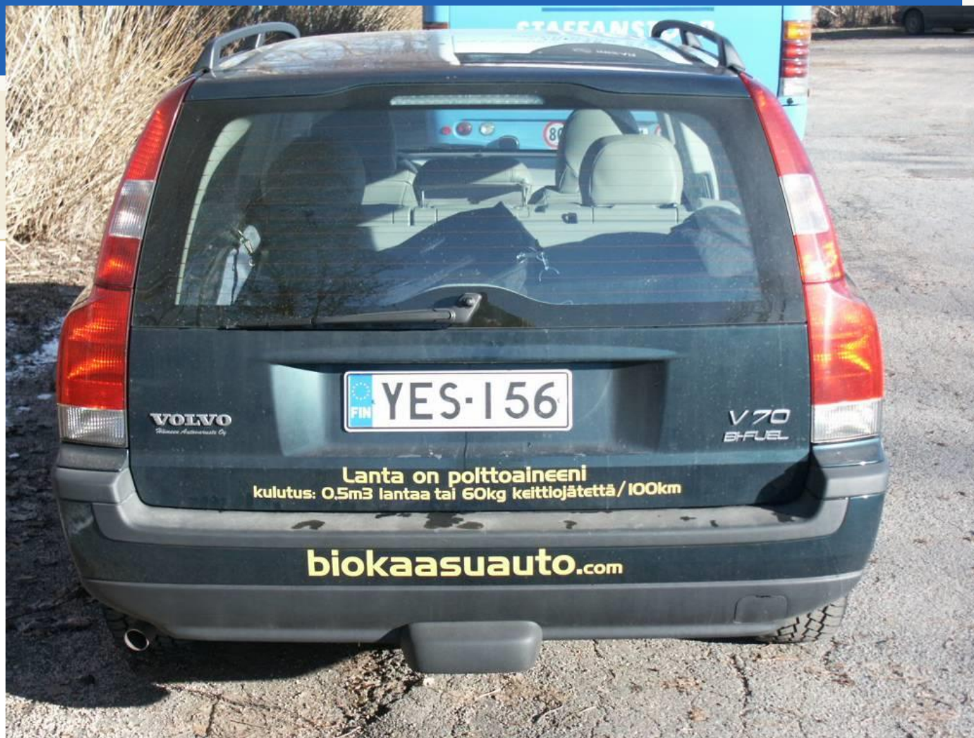
Biomethane Volvo – 0.5m 3 manure or 60kg of kitchen waste per 100km
